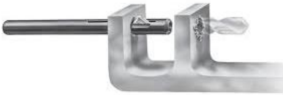
Figure 1 Deburring process with retractable cutting tools (to perform inner and outer side of a part)
